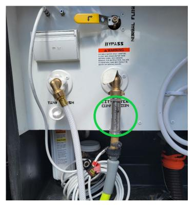
The NS-RV is so easy to install on any Recreational Vehicle (RV). Simply attach the NS-RV to your RV at the female connection for potable/city water, typically in the utility panel. Installation is possible even on older RV models without an elaborate utility panel and less space.
